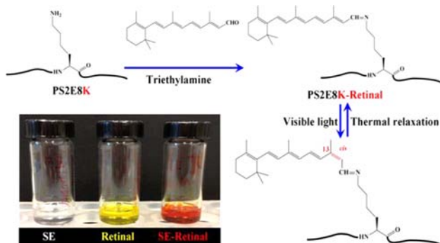
Figure 2. Schematic for retinal modification of the lysine residues in the silk–elastin copolymer PS2E8K. Insert: chemical reactions for PS2E8K before and after retinal modification (left, PS2E8K in DMSO solution; middle, retinal molecules in DMSO solution; right, retinal-modified PS2E8K in DMSO solution).
